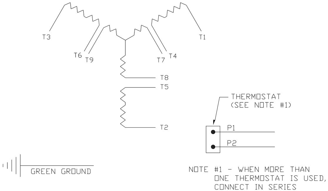
NOTE #1 - WHEN MORE THAN ONE THERMOSTAT IS USED, CONNECT IN SERIES
