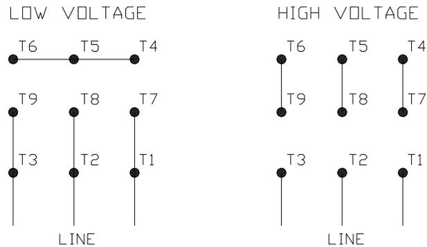
NOTE: TO REVERSE ROTATION, INTERCHANGE THE EXTERNAL CONNECTIONS TO ANY TWO LINE LEADS.
