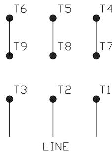
NOTE: TO REVERSE ROTATION, INTERCHANGE THE EXTERNAL CONNECTIONS TO ANY TWO LINE LEADS.
