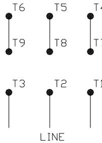
NOTE: TO REVERSE ROTATION, INTERCHANGE THE EXTERNAL CONNECTIONS TO ANY TWO LINE LEADS.
